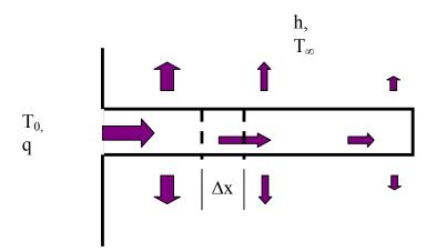
Across this segment the heat loss will be  $h \cdot (P \cdot \Delta x) \cdot (T - T_{\infty})$ , where P is the perimeter around the fin. The equivalent heat sink would be  $\ddot{q} \cdot (A_c \cdot \Delta x)$ .
