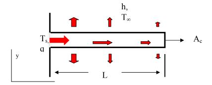
The fin is situated on the surface of a hot surface at  $T_s$  and surrounded by a coolant at temperature  $T_{\infty}$ , which cools with convective coefficient, h. The fin has a cross sectional area,  $A_c$ , (This is the area through with heat is conducted.) and an overall length, L.
